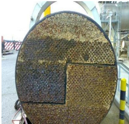
Scaling at heat exchanger Fouling at tower's infill
