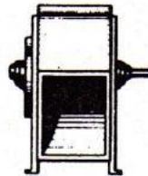
Arrangement No. 3, SW, S1 For belt drive or direct connection. One bearing on each side and supported by fan housing. Not recommended in sizes 740 diameter wheel and smaller.
